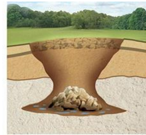
4. In weak soil, the cavity grows quickly in the shape of a funnel. In stiffer soil, such as clay, the cavity eventually becomes so large that the remaining overburden can no longer support itself or the weight of objects on the ground above it, and the overburden collapses, creating a sinkhole.
