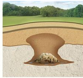
3. As this soil fills spaces in the bedrock below, a new cavity forms in the overburden, expanding toward the surface.
